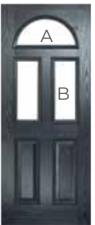
Composite Half Moon Three Radius A: 279 Glass A: 550 x 254mm Cut out B: 236 x 579mm Glass B: 207 x 550mm
